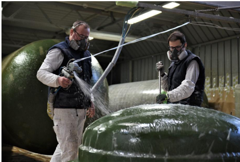
Figure2c: Chopper gun lay-up (source: internal photographic documentation TECHNOL).
