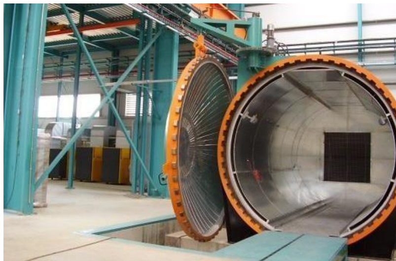
Figure 4: An example of an autoclave molding setup (source: JaviRD on Wikimedia Commons).
