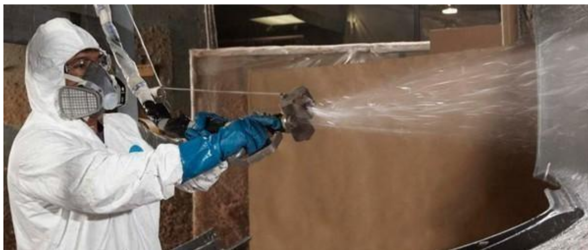
Figura 8: Lay-up of the glass fiber/resin mixture with the chopper gun (source: photo on www.graco.com ).
