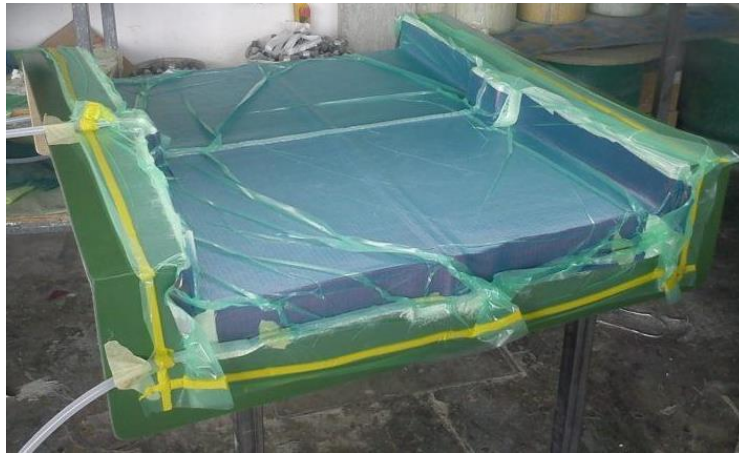
Figure3b: Preparation of a simple CFR plate by vacuum bag molding (source: internal photographic documentation TECHNOL).
