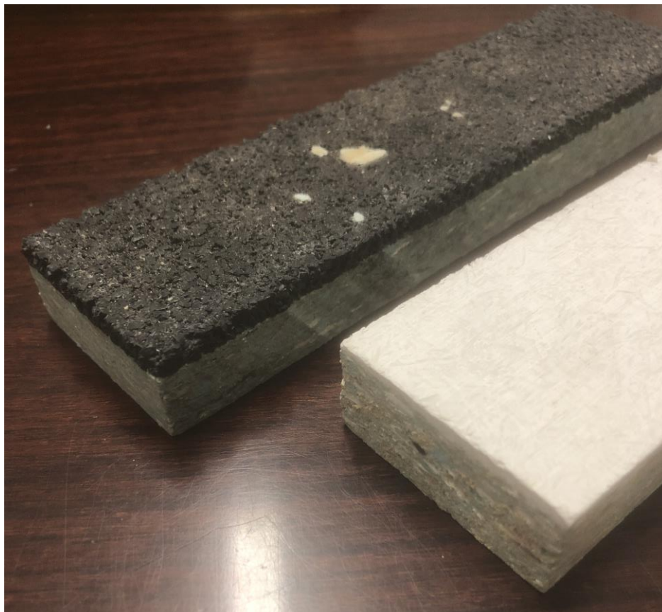
Slika 5: Levo »co-moulded« material recikliranih vlaken (RFM) in reciklirane gume, desno »co-moulded« RFM in SMC (Gees Recycling, 2020)
